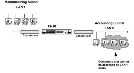
Figure 5-2 Using Filters to Restrict Access to Specific Stations
